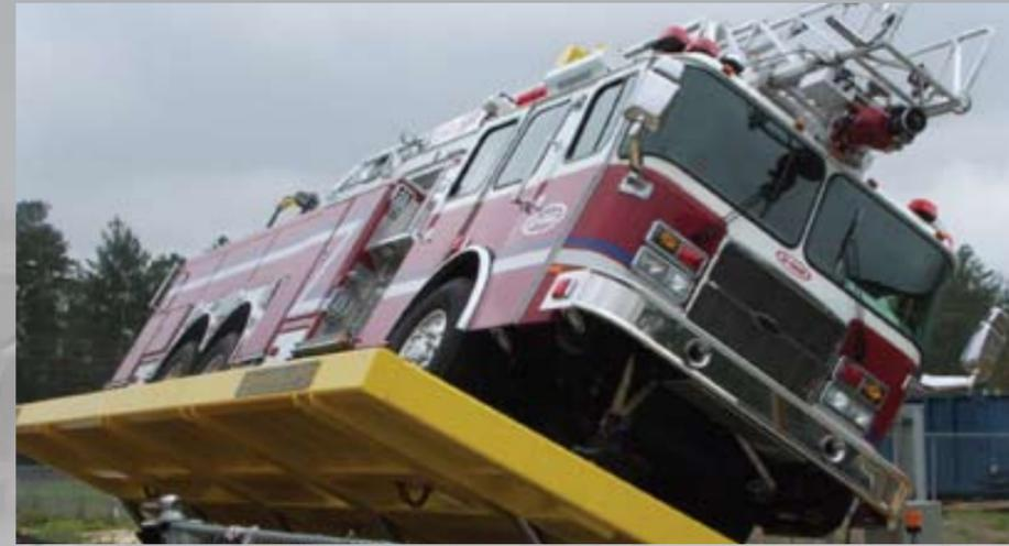
Our extruded aluminum aerial construction allows us to produce an aerial with an exceptionally low center of gravity. Combine this construction technique with our integral torque box and it results in some of the best handling vehicles in the industry.
